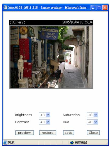
"Contrast", "Hue" and "Saturation" for video compensation. Each field has eleven levels ranged +5. In from -5 to "Brightness" and "Contrast" fields the value 0 indicates auto tuning. The user Preview press to fine-tune the image. When the image is O.K., press save to set the image settings. Restore Click on this to recall the original settings without incorporating the changes.
